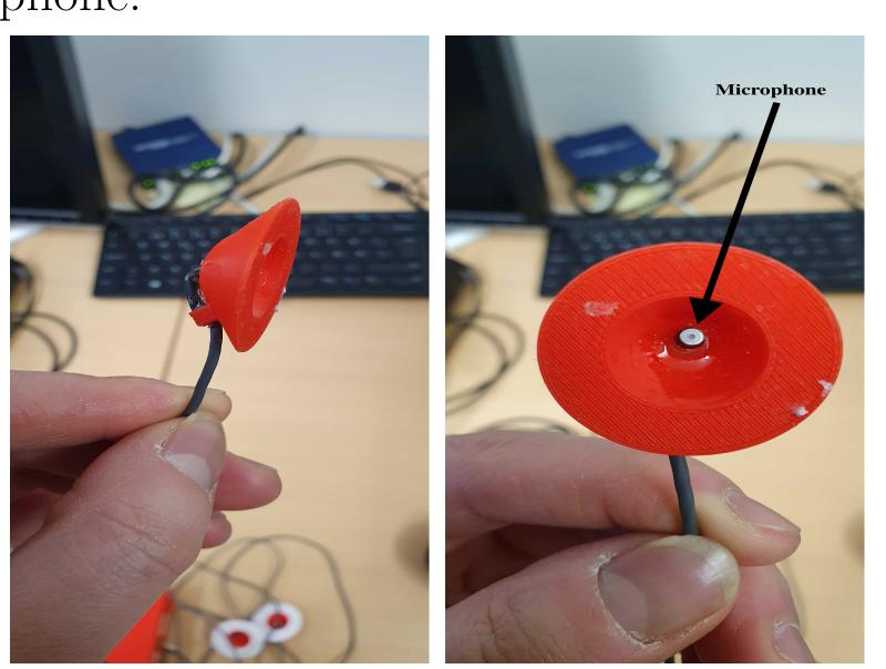
Figure 1: Cup-shaped microphones.
