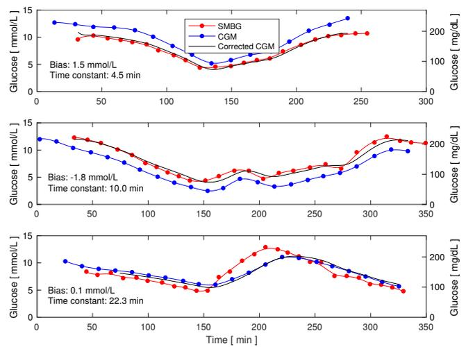
**Fig. 7.** Parameter estimation of the CGM-SMBG dynamics in three runs from the calibration sets. The three runs display different SMBG-CGM dynamics; the two first sets have clear bias effects in different directions, whereas the last set shows a clear latency effect. Biases and time constants found by the smoother are given in the plots. The black curves are bias corrected CGM signals, produced by retrieving the  $G_{isf}$  state after smoothing
