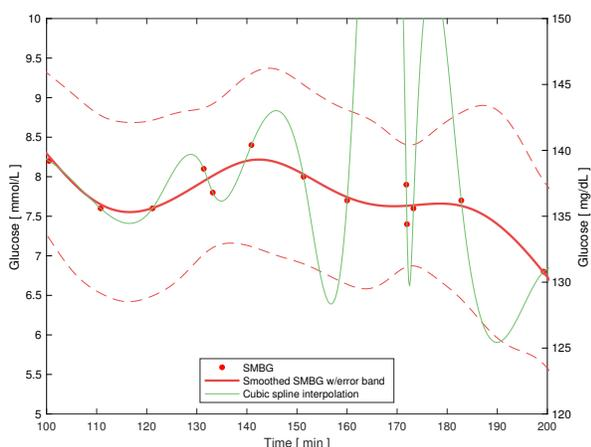
Fig. 4. Automatic handling of triplicates. The smoother estimate (red curve) goes through the mean of the triplicate measurements at  $t=172$  min. A cubic spline interpolation of the same data is shown in green for comparison, where a bad reaction to the proximity in time of the triplicate measurements is seen.
